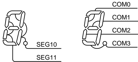
Figure 15-5 Example of COM, SEG Pin Connection (1/4 duty)
