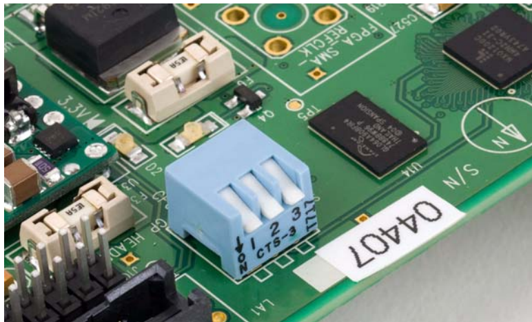
Figure 3: Configuration Mode Setting Dip Switches in “On” Position
