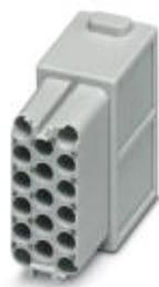
Contact insert module, number of positions: 17, power contacts: 0, control contacts: 17, Socket, Crimp connection, 160 V, 10 A, 0.14 mm<sup>2</sup> ... 2.5 mm<sup>2</sup>, application: Signal
