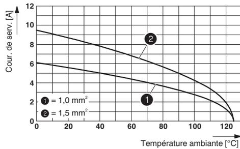
Derating diagram (3 modules in HC-B 24 housing)
