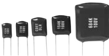
Type DLR is a radial leaded, multiple dipped with epoxy resin, polyester film/foil capacitor. The DLR boasts superior heat and humidity resistance, stable capacitance, exceptionally high value, and low cost. Because of the resulting inductance from automated single-point attachment of the leads, Type DLR is best suited for DC and low-frequency applications.
