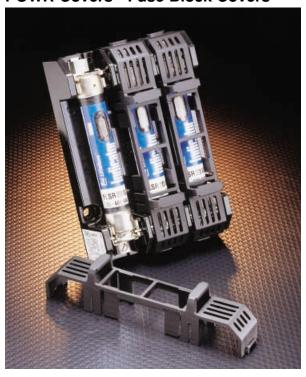
Littelfuse fuse block covers protect personnel from accidentally contacting energized contacts. Covers are available for Class H, R, J, and CD type fuses up to 100 amps.
