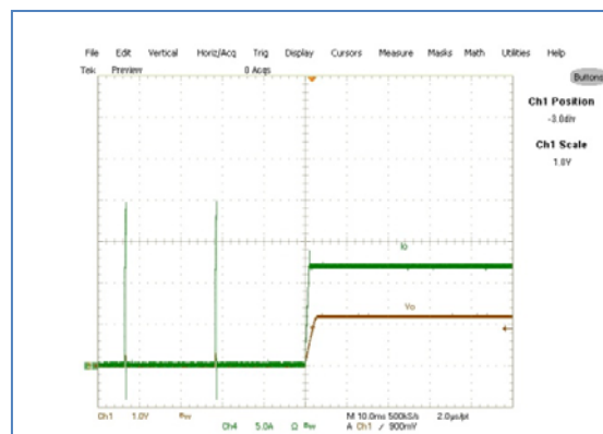
Figure 35: Short Circuit Recovery, Ch1-Vout, Ch4:Iout (5A/Div)
