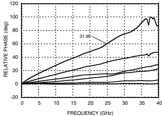
**1.0 dB LSB GaAs MMIC 5-BIT DIGITAL ATTENUATOR, 0.1 - 33 GHz**
