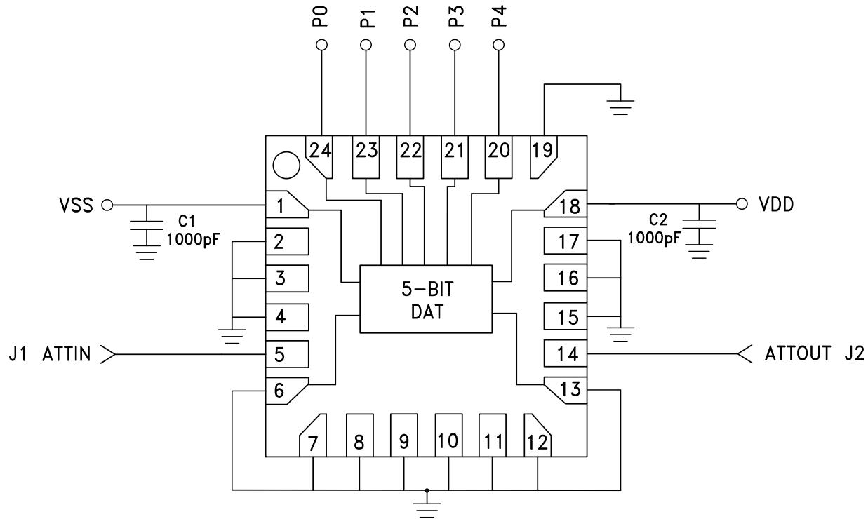
**1.0 dB LSB GaAs MMIC 5-BIT DIGITAL ATTENUATOR, 0.1 - 33 GHz**
