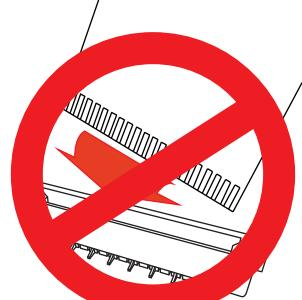
Do not keep FFC inclined when insertion
