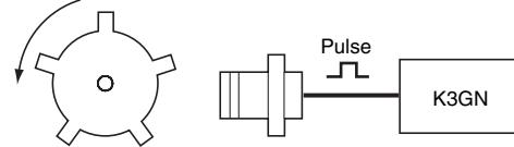
To display the rotational speed of a device that outputs five pulses per rotation:
