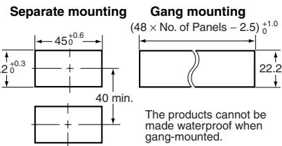
Mounting Recommended Panel Thickness 1 to 5 mm.
