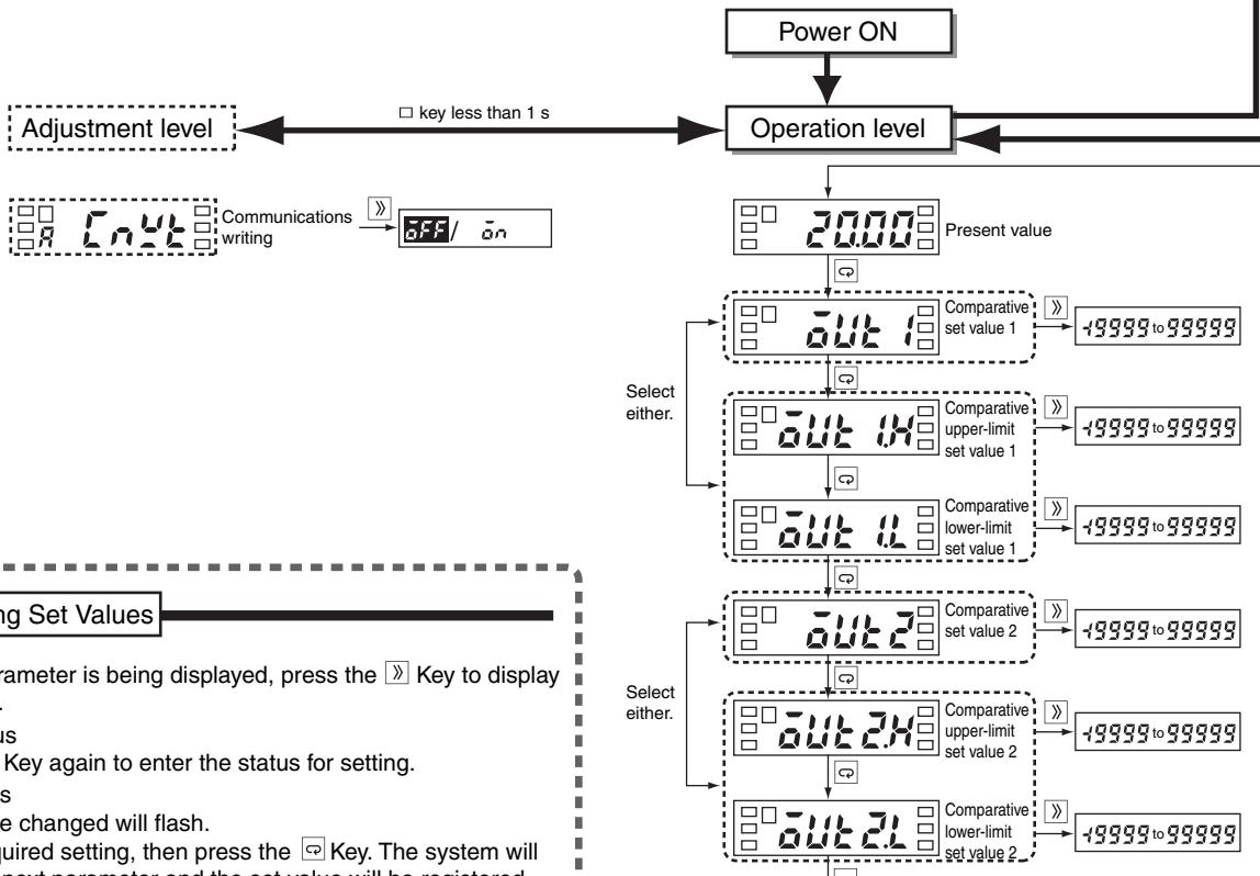
While the parameter is being displayed, press the **»** Key to display the set value.
