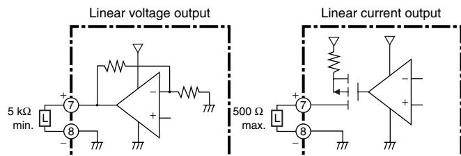
**Note:** The commons for linear output and transistor output on models with L1 and L2 are connected internally.
