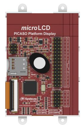
The  $\mu$ LCD-32PTU has a 3.2" TFT LCD display at the forefront of the design that showcases the power and capabilities of the PICASO processor. Combining a resolution of 240x320 pixels with 65K True to Life colours, this module is perfect for animations, slideshows and other multimedia presentations.
