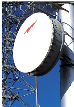
1.2 m | 4 ft High Performance, Super High XPD Parabolic Shielded Antenna, dual-polarized, 7.125–7.750 GHz, PDR84, gray antenna, enhanced white radome with flash, standard pack—one-piece reflector
