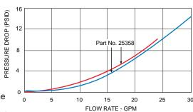
Tests conducted with units in horizontal position with water at +70°F (2 Data will vary slightly for vertically mounted units.
