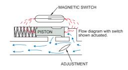
An externally rotatable vane is positioned in the main ow path within the unit. The magnet carrier piston is located in a bypass ow chamber. Pressure differential, caused by ow around the adjusting vane, displaces the spring-biased piston which actuates a hermetically sealed SPDT reed switch within the unit.
