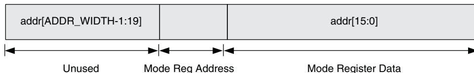
Figure 2-8. User-to-Memory Address Mapping for MR Programming
