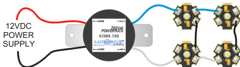
PowerPuck 2008-700 driving (4) Luxeon I LEDs from 12VDC.
