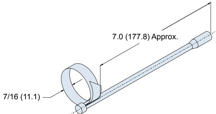
NOTE: Not recommended for composite coupling nuts (use 600-091 or 600-157)
