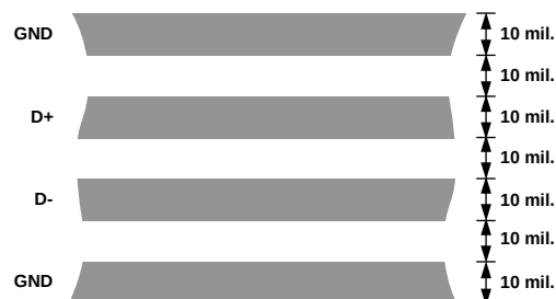
Figure 17. Arrangement of Signal Tracks
