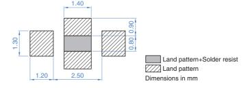
\* Make sure to connect the GND terminal of this product and the GND of the mounting circuit board by using through holes so that the distance between them is the shortest.
