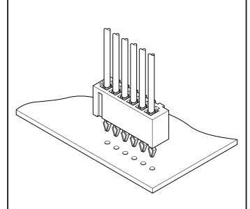
This 2.5mm pitch multi-circuit board-in connector meets the needs for high-density mounting on printed circuit boards efficiently and economically. The connector can be used for VCRs, car stereo systems, audio products, and many other consumer-oriented electronic products.
