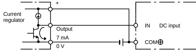
NPN open-collector output
