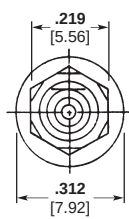
Receptacle, Front Mount Part Number 145-0002-0001
