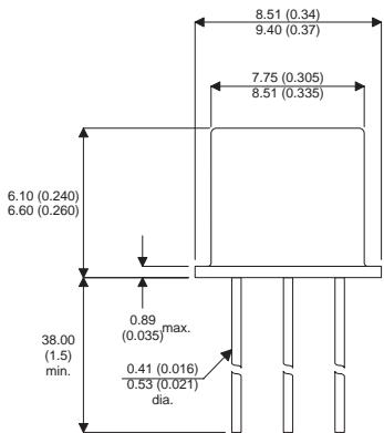
**Bipolar NPN Device in a
