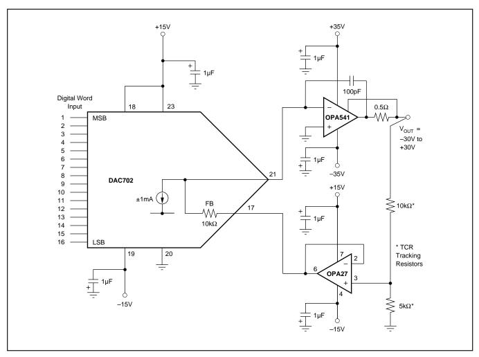
FIGURE 7. 16-Bit Programmable Voltage Source.
