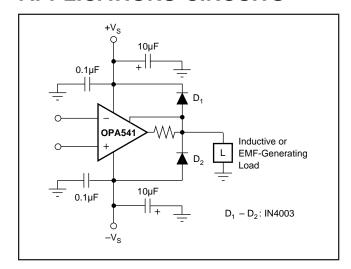
FIGURE 2. Clamping Output for EMF-Generating Loads.
