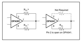
FIGURE 4. Isolating Capacitive Loads.
