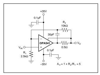
FIGURE 5. Paralleled Operation, Extended SOA.
