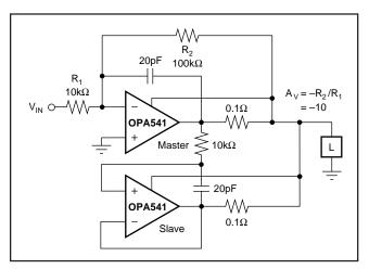
FIGURE 3. Replacing OPA501 with OPA541.
