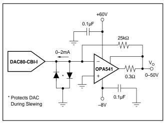
FIGURE 6. Programmable Voltage Source.
