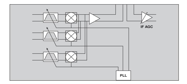
The BCM3418 is a complete QAM Digital Cable Tuner-on-a-chip that supports both 64- and 256-QAM applications. The BCM3418 utilizes a highly integrated version of the single conversion architecture. The input signal is split into three bands, each with a variable bandpass filter and mixer, controlled by a two-wire serial bus that is MBus compatible. The IF amplifier
