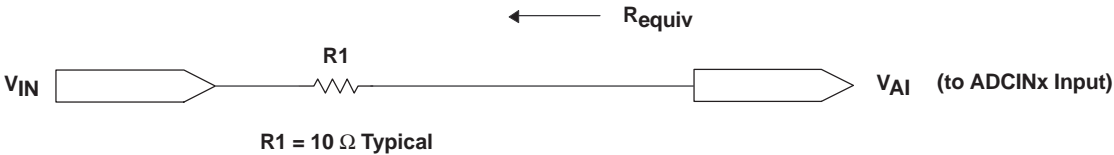
Figure 41. Typical ADC Input Pin Circuit
