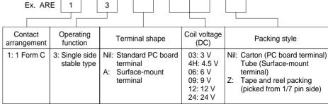
Note: Tape and reel packing symbol "-Z" is not marked on the relay.
