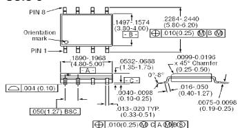
8- Lead SOP outline dimensions Narrow body .150 (All dimensions per JEDEC No. MS-012-AA, Issue C) Dimensions in ( ) are in mm.
