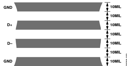
Figure 20. Arrangement of Signal Tracks
