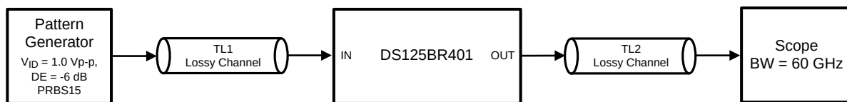
Figure 10. Test Setup Connections Diagram
