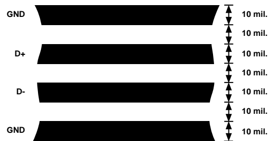
Figure 19. Arrangement of Signal Tracks
