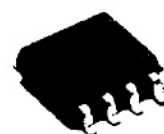
Outline 8P2S-A(FP) 1.27mm pitch 225mil SOP (4.4mmx5.0mmx1.5mm)
