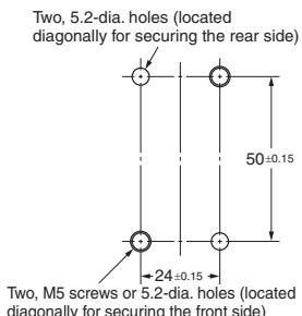
Only the HL-5□□□G has M5 x 0.8 (10 depth min) screw holes on the rear side.
