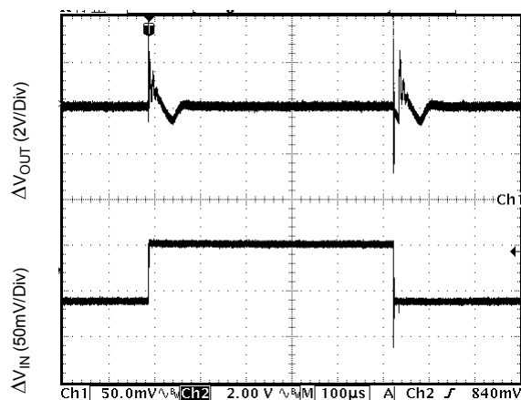
Figure 24. Line Transient Response (Conditions: V_{IN}=2.5V to 5V , V_{OUT}=0.8V , I_{OUT}=10mA , C_{IN}=0\mu F , C_{OUT}=2.2\mu F )
