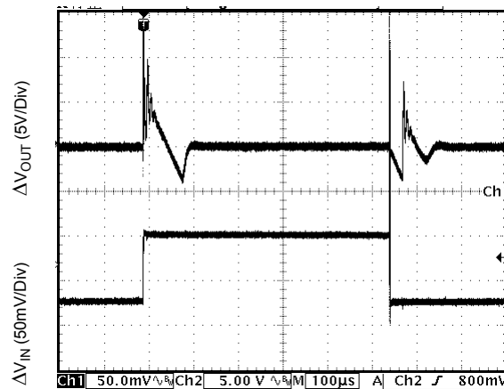
Figure 25. Line Transient Response (Conditions: V_{IN}=2.5V to 10V , V_{OUT}=0.8V , I_{OUT}=10mA , C_{IN}=0\mu F , C_{OUT}=2.2\mu F )
