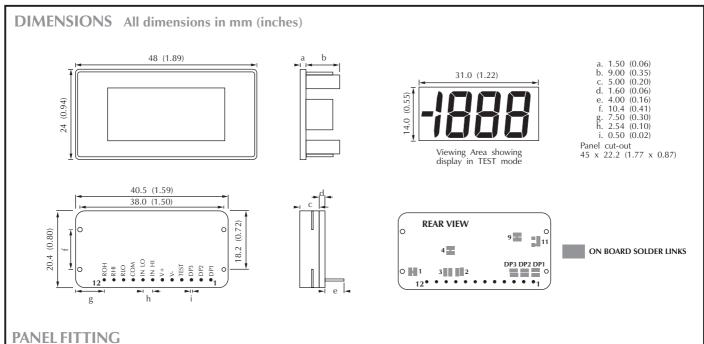
Fit the bezel to the front of the panel and then locate the meter into the bezel from behind. Alternatively the meter and bezel may be assembled before fitting into the front of the panel but care must be taken not to use excessive force. Finally fit the window into the front of the bezel.
