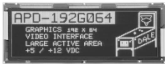
The APD-192G064-1 has been designed to offer high brightness and superior viewing aesthetics in a package that is very affordable. This display is ideal for low to medium level information content messages and would be ideal for applications such as arcade games, process control, POS terminals, medical equipment, message centers and ATM machines.
