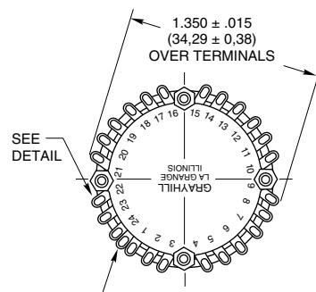
Note: Common location for a single pole per deck switch. For common location on multipole switches see circuit diagrams.
