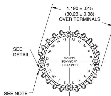
Note: Common location for a single pole per deck switch. For common location on multipole switches see circuit diagrams.
