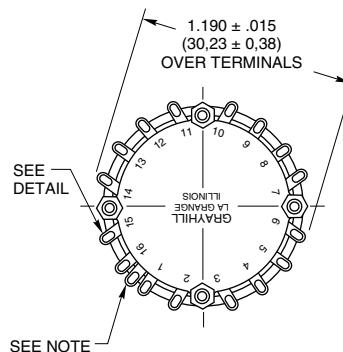
Note: Common location for a single pole per deck switch. For common location on multipole switches see circuit diagrams.
