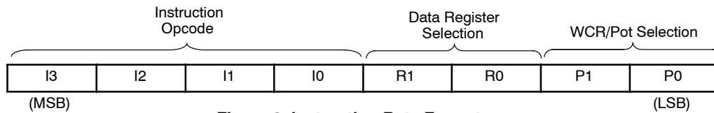
Figure 9. Instruction Byte Format
