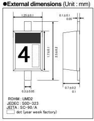
●Lead size figure (Unit : mm)
