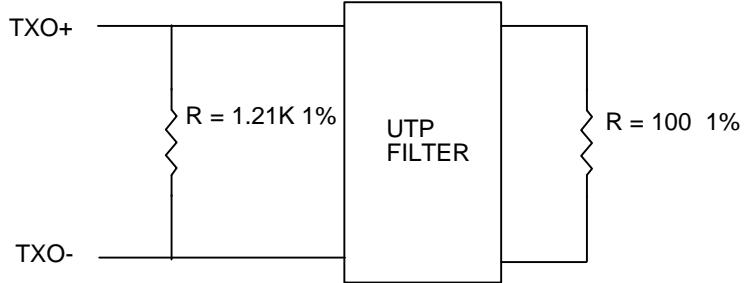
Note: In the above diagram, the UTP filter used for all testing is a Valor FL1012.
