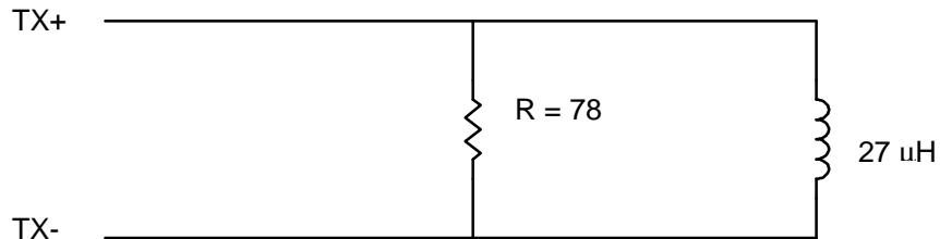
Note: In the above diagram, the TX+ and TX- signals are taken from the AUI side of the pulse transformer. The pulse transformer used for all testing is a  $100\mu\text{H} +/-0.1\%$  Pulse Engineering PE64103.
