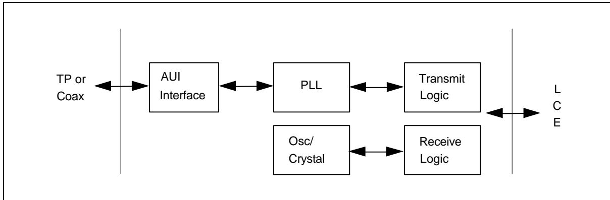
The Manchester encoder/decoder handles code interpretation between NRZ signals and Manchester coded signals. The PLL locks the receiving signals with an internal voltage control oscillator (VCO) so that network noise can be eliminated before the signals enter the core coprocessor. The collision decoder detects whether a collision has occurred on the network. The oscillator logic supplies the PENTIC+ with the required 20 MHz clock. This clock also supplies the SNA clocking system.
