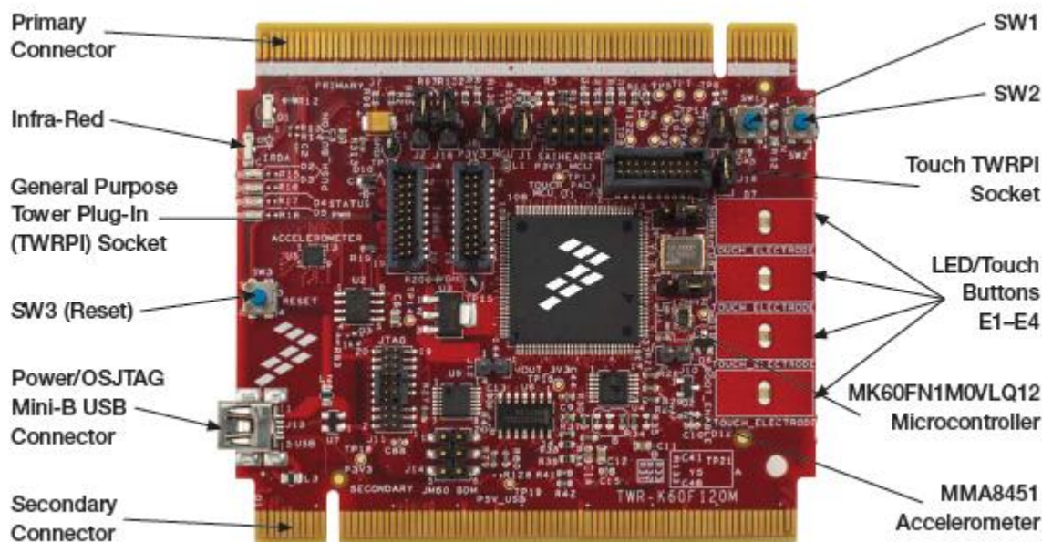
Figure 2. Callouts on front side of the TWR-K60F120M
