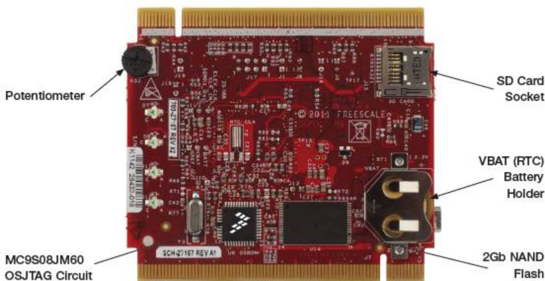
Figure 3. Callouts on back side of the TWR-K60F120M
