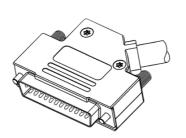
Place the assembly into the hood half as shown
