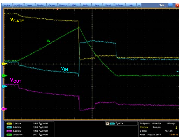
Figure 6. Output Short Circuit Zoom In
