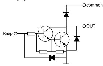
The 'common' pin is, as the name states, common for all open collector drivers. It is not connected to any other point on the Gertboard. For more details see the datasheet of the ULN2803a.
