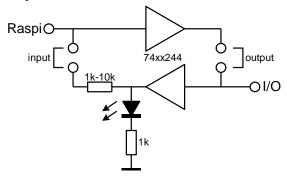
In order to make the port function as input you have to place the 'input' jumper.
