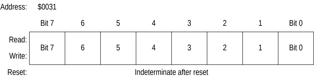
Figure 11-21. TIMA Channel 3 Register Low (TACH3L)
