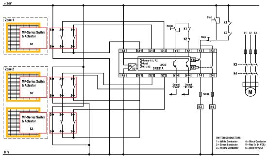
The MF Series switch and actuators are integrated with an SR131A safety monitoring relay. The safety contacts of the MF switches for zone 2 are wired in Series/Parallel. This method allows multiple gates or switches to be wired to a single channel on the safety monitoring relay or control unit.
