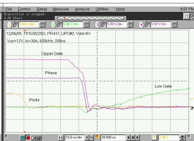
Figure 9-2. Phase Falling-Edge Switching Waveforms (10 ns/div) of the Power Stage in Figure 7-1
