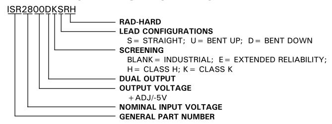
The above example is a Class K adjustable dual output rad-hard converter
