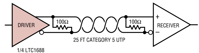
Figure 12. 100Mbps Differential Data Connection
