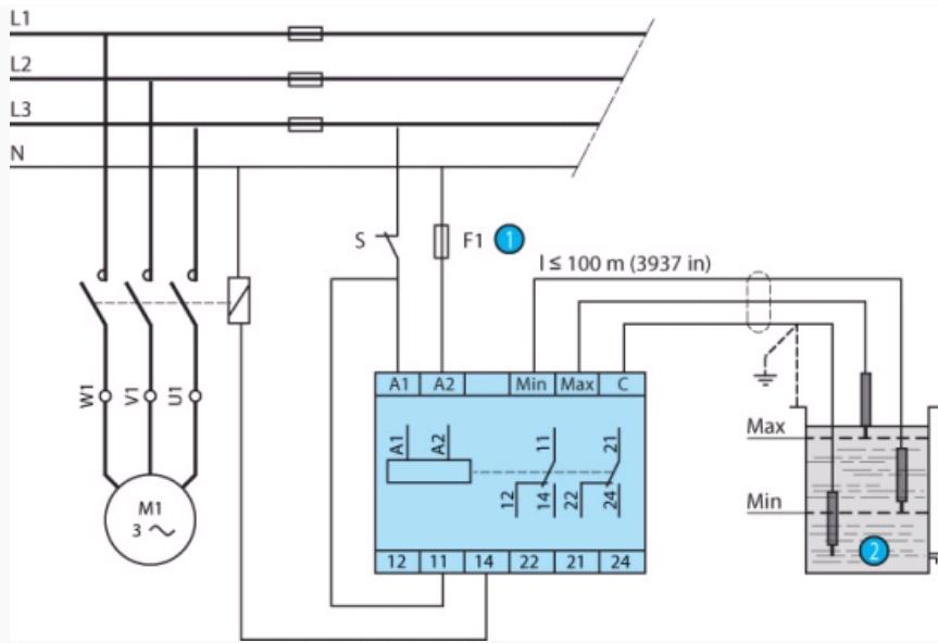
NB : Probe cable : screened cable recommended, screening and "common" connected to earth. The probe cable does not have to be screened, but it is inadvisable to mount it close to the power cables. For mono level, use the "com" and "min." electrodes.
