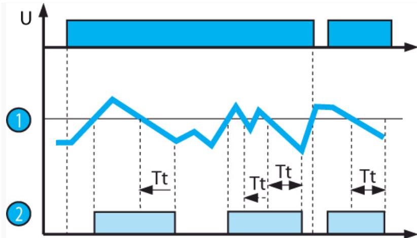
**One-level control (min. probe), emptying function, off-delay**
