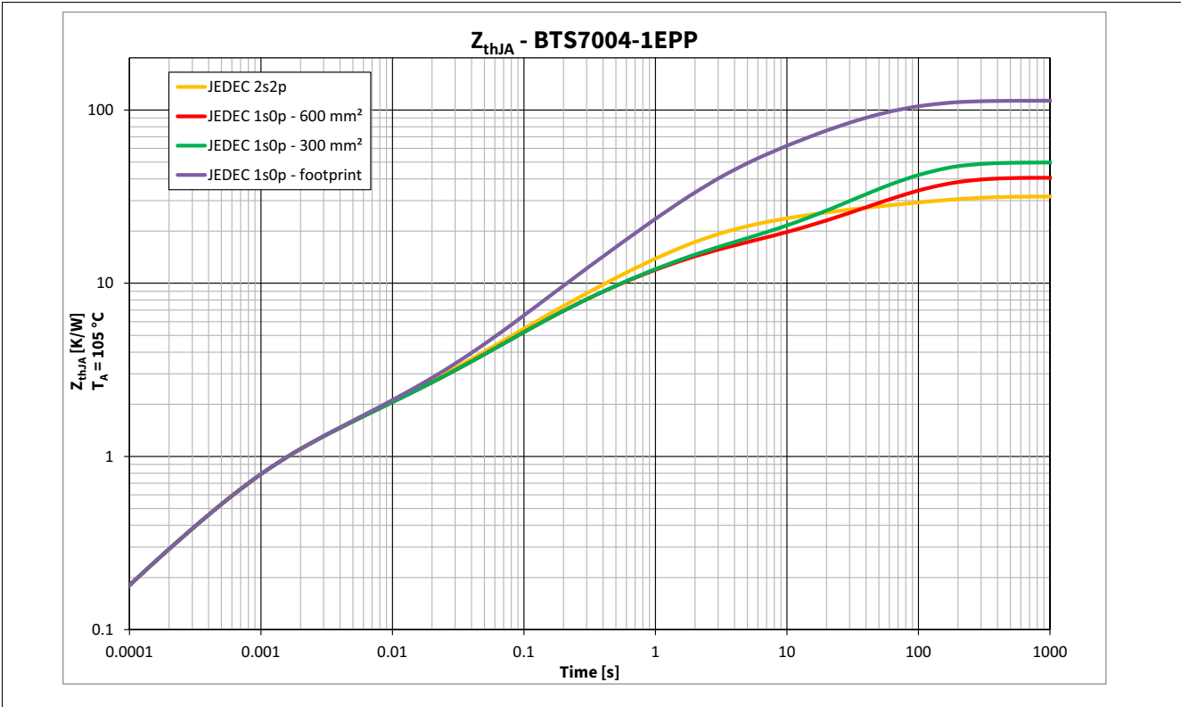
Figure 9 Typical Thermal Impedance. PCB setup according Chapter 4.4.1
