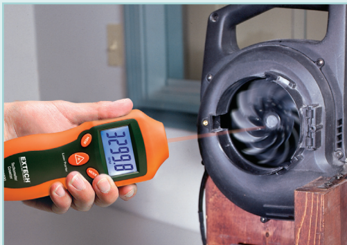
Non-contact fan blade RPM or REV testing
